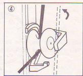
Thread two yarns of different colours through the Auto-Tension in the following order.
