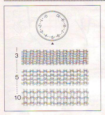
The Stitch Dial is operated to regulate the size of stitches by setting its number to the A mark at the front of the Stitch Dial.
