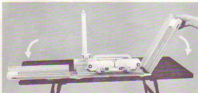
4. Hold the ends of the needle bed and gently lay down flat on the table.
