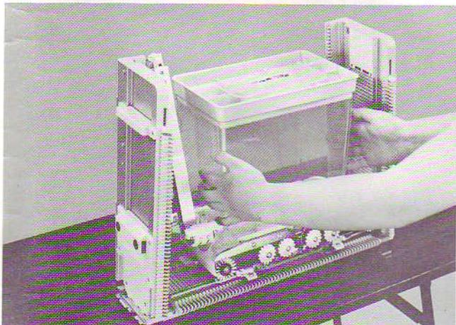
9. Replace the utility box to the original position, and place the case cover over it.
