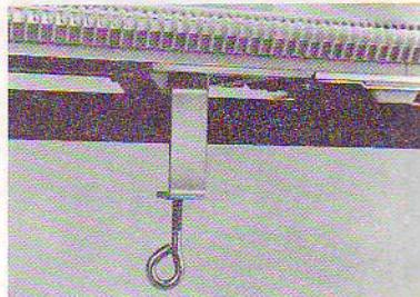
7. Stretch the Tension Post straight, and push in till it locks in position.
