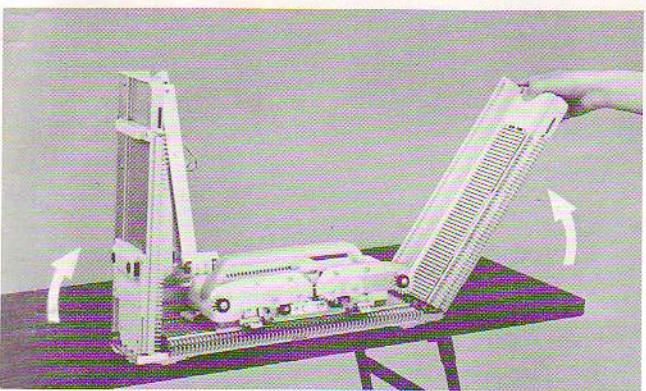
8. Fold up both ends of the needle bed till they stop in locked position.
