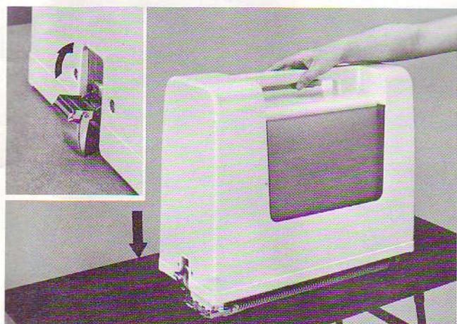
10. Lock the latch at both sides of Case Cover.
