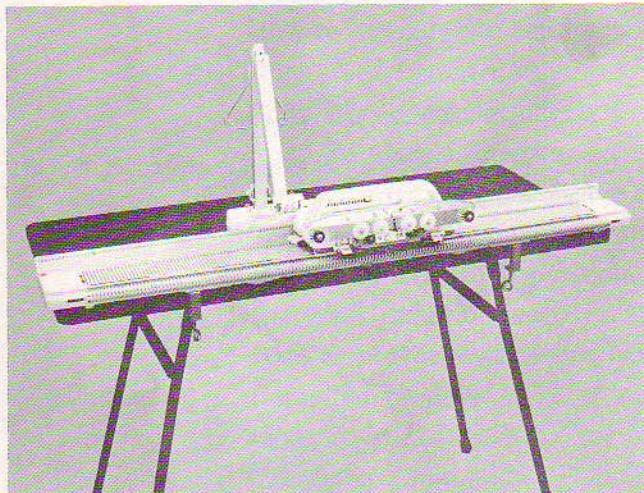
6. Take out two Clamps from the accessory box, and fix the machine as shown on the table.
