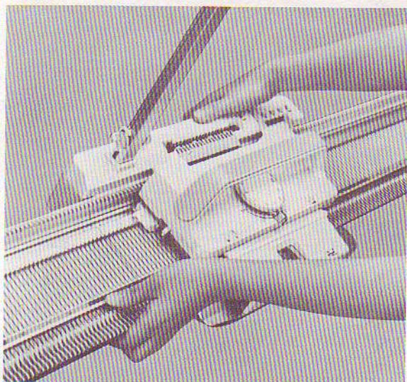
If you carry the machine as it is opened, hold centre portion of the needle bed.
