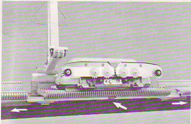
7. Press the Red Button (Lock Lever Button) at the front bottom edge of the needle bed.
