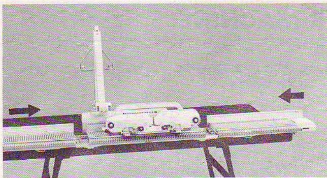
5. Push in both ends of the needle bed till they lock in position with a clicking sound.
