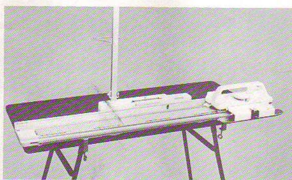
To use the machine, secure it with Clamps on the table.
